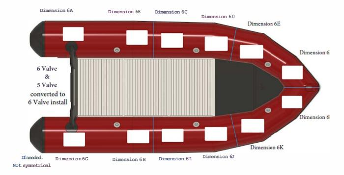
The above diagram represents a 6 valve or 5 valve converted to a 6 valve boat. Dimension  $6G \cdot 6L$  are used if non-symmetrical. If none equals SAME as PRT.
